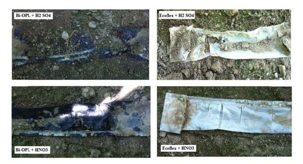
Fig. 5: The bioplastics degradation after the exposure time at field
