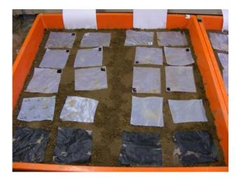
Fig. 1: Bioplastic strips are placed on the soil surface in plastic griddle.
